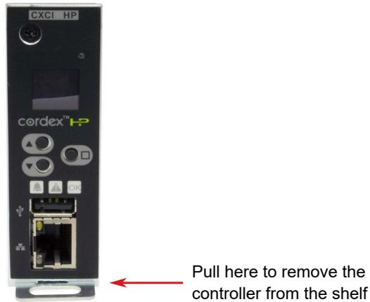
**⚠ CAUTION:** When removing the controller in a live system that has an LVD, ensure that the LVD override jumper is set to correct position to avoid possible service disruption. Refer to the wiring and connections section of the manual and the connection drawings.
