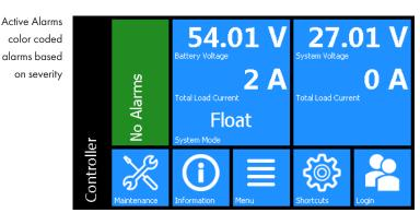
System Status Single or dual panel options: system signals and system mode (DC and converter systems shown)
